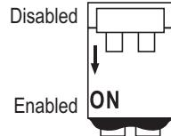
**Note:** If an external termination connector is used, the switch must be in OFF position.
